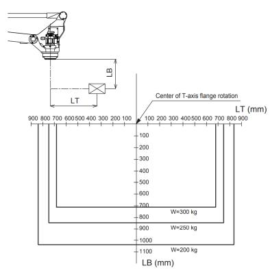
Depending on the Cg the robot will either be able to carry the rated load or less or non...if the tool Cg is too far from the robot's flange.
